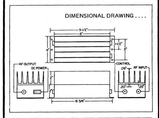
PLEASE NOTE . . . . All rated amplifier outputs are measured under laboratory conditions with a proper drive level. If the amplifiers are operated with improper drive, at a voltage less than 13.8 VDC, with mismatched cables, or with a mismatched antenna the output will be less than maximum!
